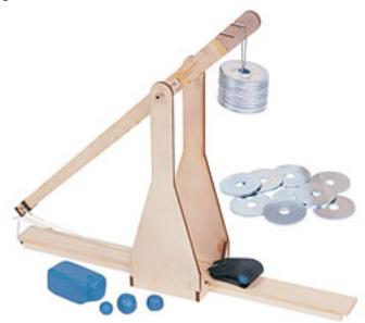
We want to examine the effect of rope length and amount of weight on the distance that a projectile will fly. The treatments in this experiment are the combinations of weight (number of washers, 3, 5, 7, or 9) and length of "rope" (7, 8, 9, or 10 inches). The response is the distance in inches that the trebuchet will throw a small ball of putty. There are 48 runs, three for each of the factor/level combinations in random order.
